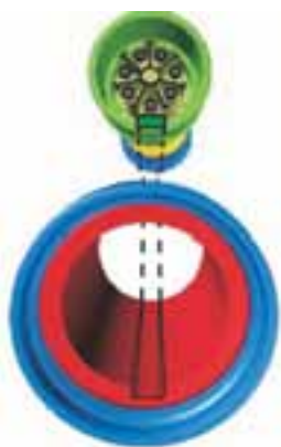
Fig. 7.4 Fit plug insert
