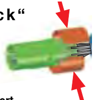
Fig. 14.5 Fit divided insulating sleeve
