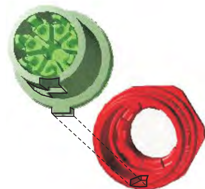
Fig 10.3 Assembling receptacle insert
