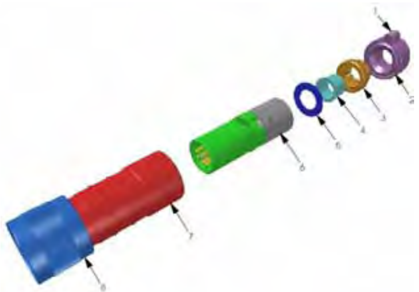
Fig. 12-1 Plug with cage clamp terminals (plastic/ metal)
