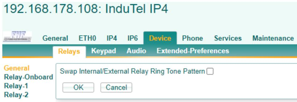
**Figure 6. Device-specific relay settings**
